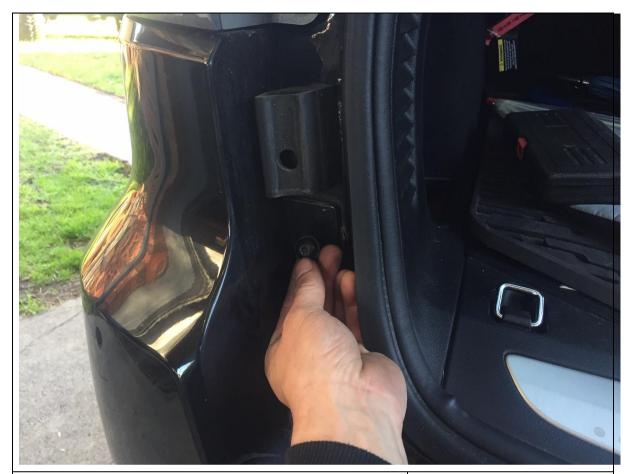
1. Open tail gate and remove screw with T30 Torx bit shown on LH and RH side.
