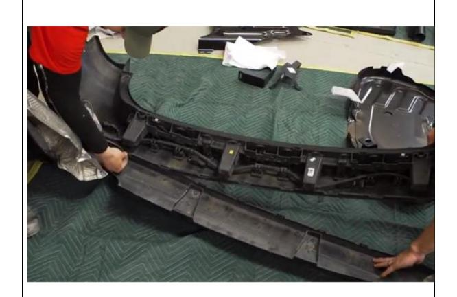
14. Split lower section of bumper from upper section. Use pry tool, flat head screw driver and T20 Torx bit
