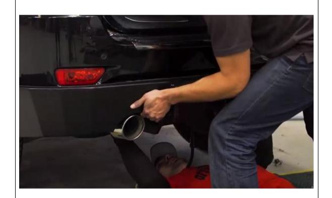
17. With the help of that friend of yours, lift the bar onto the vehicle while one lies underneath and starts all the bolts.
