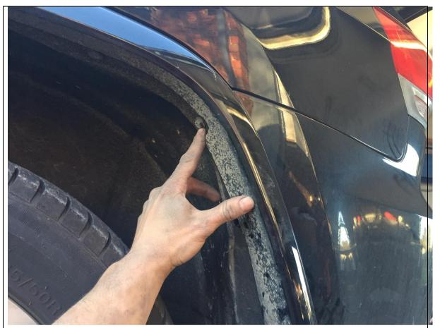
6. Remove screw with 10mm Socket or spanner, repeat for other side.
