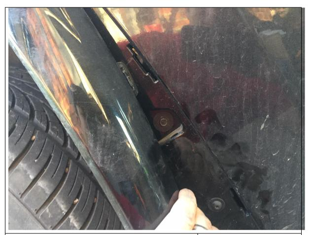
5. Remove Small bolt shown in middle, repeat for other side. Use 7mm spanner or socket
