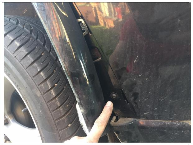
4. Peel back flare and remove small screw with T20 Torx bit behind. Repeat for other side.
