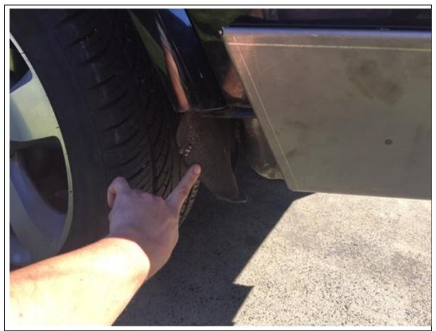
22. Trim felt liner to suit new bar with box cutter.
