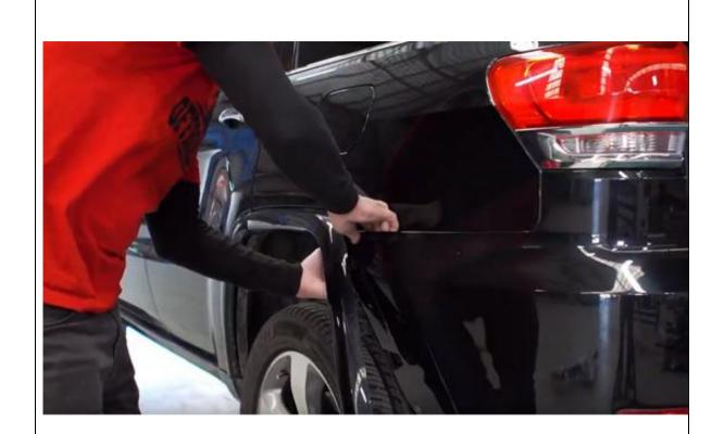
7. Pull flare aside with use of flat screwdriver on each clip to release from body. Repeat for other side.
